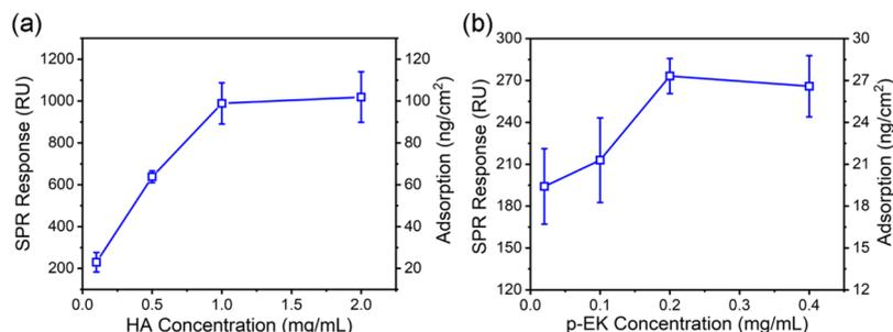
**Figure 5.** (a) SPR response and the corresponding adsorption of HA solution with different concentrations on the Au surface, (b) SPR response and the corresponding adsorption of zwitterionic p-EK peptide solution with different concentrations on the HA-modified surface.
