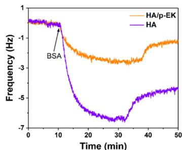
**Figure 4.** QCM sensorgram of 1 mg/mL of BSA solution on the HA-modified Au surface and HA/p-EK-modified Au surface.
