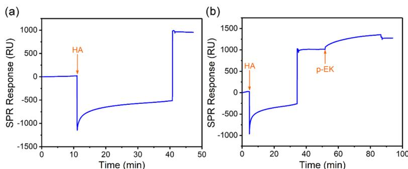
**Figure 1.** SPR sensorgram showing the modification progress of (a) thiolated HA on Au surface and (b) thiolated HA together with zwitterionic p-EK peptide on Au surface.
