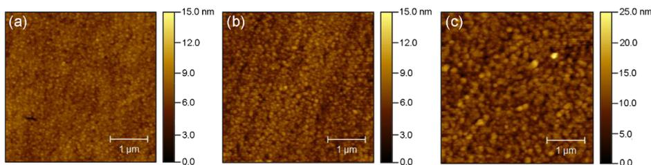
**Figure 3.** Surface morphology of (a) Au, (b) Au-HA, and (c) Au-HA/p-EK substrates.
