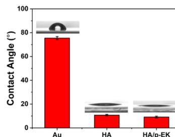
**Figure 2.** Water contact angle of Au, Au-HA, and Au-HA/p-EK surfaces.
