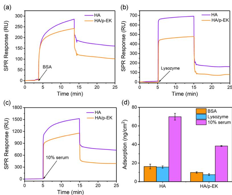
**Figure 6.** SPR sensorgrams of (a) 1 mg/mL of BSA, (b) 1 mg/mL of lysozyme, and (c) 10% human serum on HA- and HA/p-EK-modified Au surfaces, (d) nonspecific adsorption amount of protein on HA- and HA/p-EK-modified Au surfaces.
